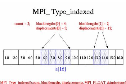
MPI Type indexed(count, blocklengths, displacements, MPI FLOAT, &indextype);
